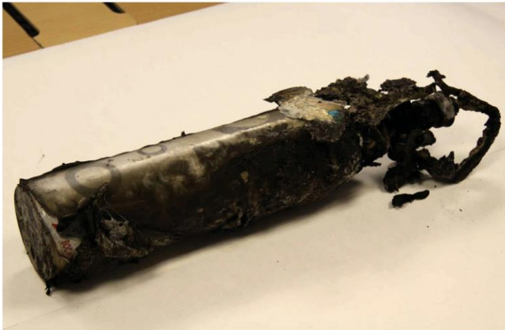
Figure 1 The remains of the burnt oxygen cylinder. Published with permission from Anaesthesia . 1
